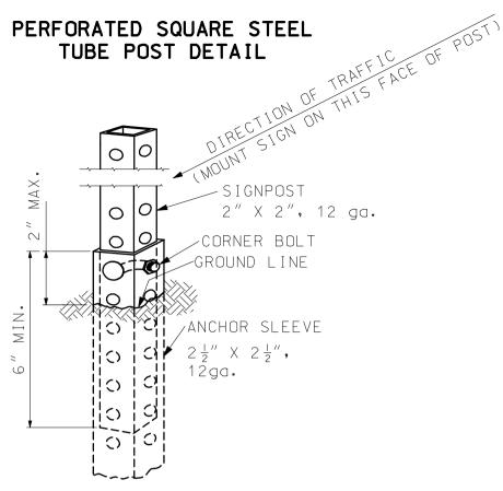
THE SIGNPOST IS ATTACHED TO THE ANCHOR SLEEVE WITH THE CORNER BOLT PER MANUFACTURER'S SPECIFICATION.
