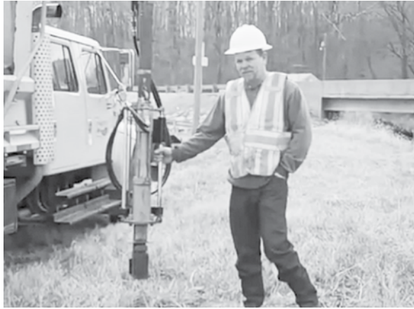
Senior Maintenance Worker Todd McGregor explains that the Channel Driver speeds up the driving process and improves safety.
