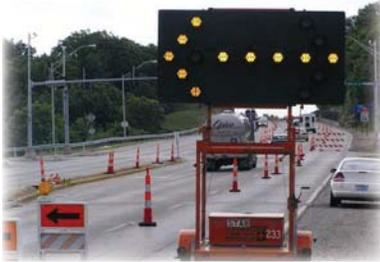
The overall minimum dimensions of the panels are 60 in. wide x 30 in. high for truck-mounted units and 96 in. wide x 48 in. high for trailer-mounted units. Panels for both units shall include 15 yellow elements.
