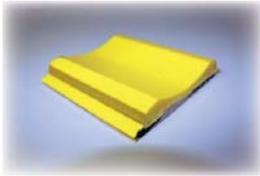
These markers, available in white and yellow, are typically **used to temporarily mark changes in normal roadway use by applying them to the road surface at 40-ft. intervals**. This spacing may be reduced by one-half when marking intersections, ramp gores and other transition areas.
