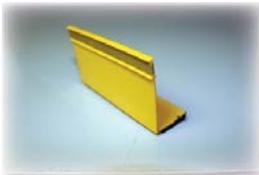
with a retroreflective sheeting on both faces of the vertical article and a pressure-sensitive adhesive on the base. These markers, available in white and yellow, are typically **used to temporarily mark centerlines and lane lines by applying them to the road surface at 40-ft. intervals** prior to or after, depending on the type of surface treatment, an operation and removing the protective film
