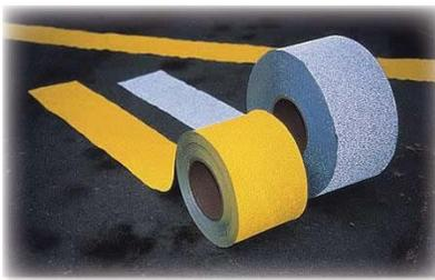
retroreflectorized tape with a pressure-sensitive adhesive on the back. The tape, available in white and yellow, may be used to provide a surrogate permanent pavement marking or it may be cut into 4-ft. long articles and applied to the road surface at 40-ft. intervals as a temporary pavement marking. The length and spacing of the latter pavement marking may be reduced by one-half when marking intersections, ramp gores and other
