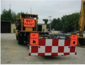
Truck-mounted attenuators are energy-absorbing devices attached to the rear of trucks used as protective vehicles. These devices are designed to protect the motorist and protective vehicle driver upon impact.
