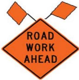
Temporary traffic control signs convey, in words and symbols, both general and specific messages used by motorized and non-motorized traffic to navigate the temporary traffic control zone safely and efficiently.
