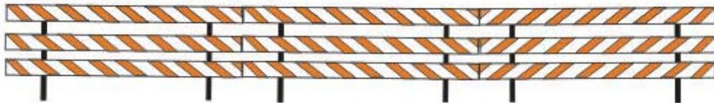
(Typical installation of Type III Barricade with 12' lane no shoulder)
