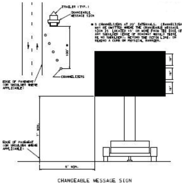
**Channelizers may be omitted** where the CMS is located 15' or more from the edge of any shoulder (edge of roadway where there is no shoulder), beyond the ditch line, or behind a curb or physical barrier.
