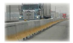
Due to the amount of resources needed to put barrier in place, this option is generally reserved for long-term stationary operations where the need for the noted function is critical.
