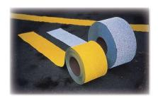
retroreflectorized tape with a pressure-sensitive adhesive on the back. The tape, available in white and yellow, may be used to provide a surrogate permanent pavement marking or it may be cut into 4-ft. long sections and applied to the road surface at 40-ft. intervals as a temporary pavement marking. The length and spacing of the latter pavement marking may be reduced by one-half when
