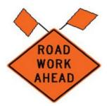
Temporary traffic control signs convey, in words and symbols, both general and specific messages used by motorized and nonmotorized traffic to navigate the temporary traffic control zone safely and efficiently.
