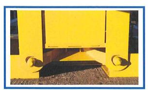
GOOSENECK: Air activated lock. PTO operated hydraulics. Hydraulic neck support arm. NOTE: All hydraulics are set to operate at 3,000 PSI.
