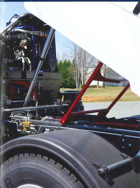
ABOVE Stainless steel hydraulic lines, wider blower intakes, and new improved body safety prop automatically deploys.
