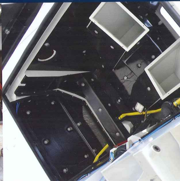
New standard engine cowl sound suppression.
