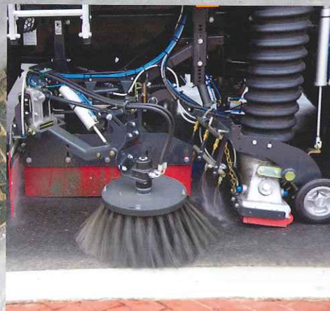
Variable lateral control Varibrush option.
