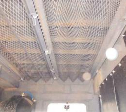
Saw Tooth Screens: Increased screen surface area eliminates the need for a screen vibrator and lowers cost of operation PM 10 Certified: Meets AQMD 1186 requirements to pick up and contain harmful particulates
