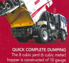
steel walls, a ¼ inch (6.35 mm) thick steel floor with easy dropdown screens for quick cleanup. A 50 degree tilt angle ensures efficient dumping. Hopper controls are safely accessible on the curb side of the sweeper and conveniently located in-cab for quick unloading of the hopper.
