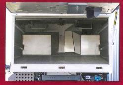
STAINLESS STEEL HOPPER SYSTEM This complete hopper body is constructed entirely of 304 grade stainless steel to provide maximum service life, even in the most corrosive applications.
