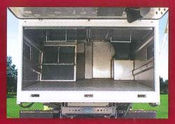
This complete hopper body is constructed entirely of 304 grade stainless steel to provide maximum service life, even in the most corrosive applications.
