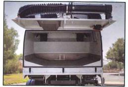
STAINLESS STEEL CONSTRUCTION High quality materials such as 304 Grade Stainless Steel are integrated into the **8.5 Cu.Yd. Hopper.**
