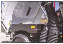
The twin water tanks provide a total tank capacity of **500 gal.**
