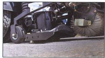
The **V-shaped Suction Nozzle** with its large aperture, made of 4 mm steel, conveys the swept material directly into the suction tube. This design enables the **Global V6** to lift the Heaviest of debris in any application.
