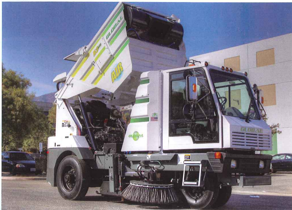
DUST SUPPRESSION SYSTEM consists of 230 Gallon Water tank & (2) Two Water Pumps rated at 3.5GPM @ 45Psi.
