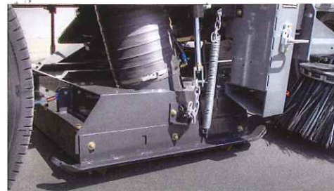
The Sweeping system consists of 72" Wide Pick-Up Hood with Carbide Dirt Shoes, and Large 47" Digger-Type Gutterbrooms. Combining both with a Large 32" Suction fan equals to one of the most powerful AIR Street Sweepers available today.
