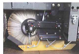
ABOVE Polyurethane Dirt Shoes will never damage while sweeping and last well above 1000 hours
