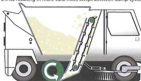
BELOW Elevator Type: 11 Flight squeegee with replaceable corded rubber tips; Continuous molded rubber belts. Hydraulic Motor: Direct drive: Variable Forward and Reverse; Displacement - 15.8 cu. in./rev. 5.6 cu/yd hopper capacity compared to 3.5 cu/yd for competitive machines resulting in more curb miles swept between dump cycles.
