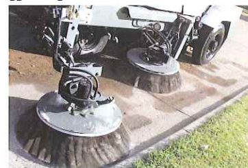
ABOVE Optional Front Articulating brush allows for extra reach to shoulders and center islands. Via In-cab joystic, the articulating front brush can be positioned on left or right side allowing for sweeping on right or left without changing seating positions.
