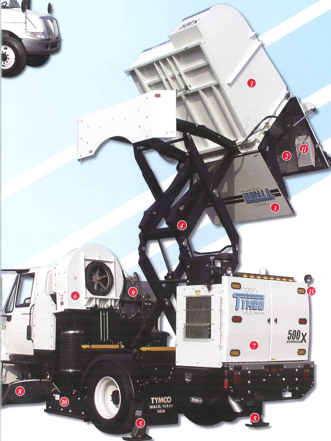
The Tilt-N-Seal™ blower system ensures long seal life between the hopper and blower housing.
