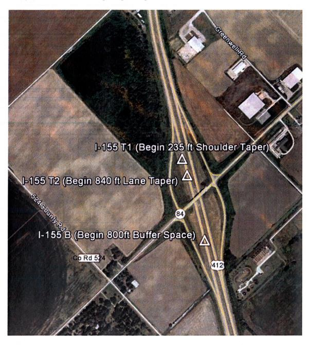
The Work Zone Signing leading into the Lane and Ramp Closure (TA-33 with Speed Reduction to 60 mph) (TA-44 used at entrance ramp)
