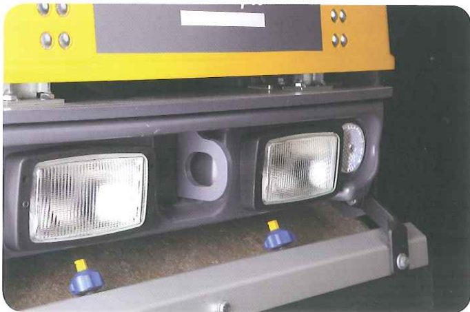
Pressurized sprinkler system with a powerful water pump and self-draining sprinkler tubes and nozzles.
