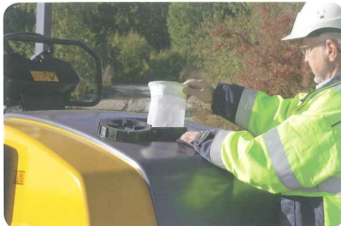
The water tank has a large opening for easy filling.
