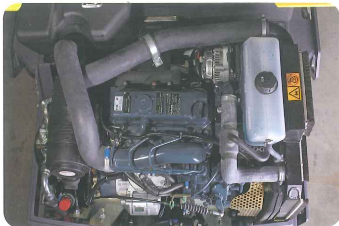
Silent and powerful water-cooled Kubota diesel engine. The large easy-to-open engine hood contributes to great accessibility.
