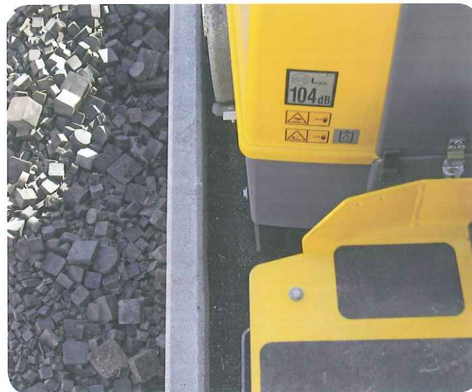
High clearance of the edge of the drums facilitates compaction close to high curbstones. Excellent view over the drum edges for better control and compaction results.
