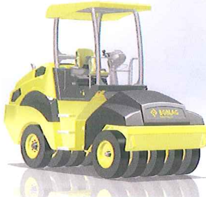
Center swivel seat provides excellent comfort and visibility in both travel directions
