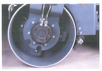
Big drum diameter makes compaction easier even on soft tricky asphalt mixes. Thick drum shells for long life.
