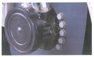
Fail safe brakes on both drums (or drum + combi wheels) which apply automatically in the event of failure in engine, hydraulics or electrical fault in the brake system.
