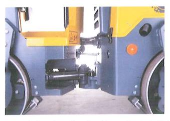
Long service intervals together with maintenance free steering hitch and steering cylinder contribute to a minimum of maintenance.
