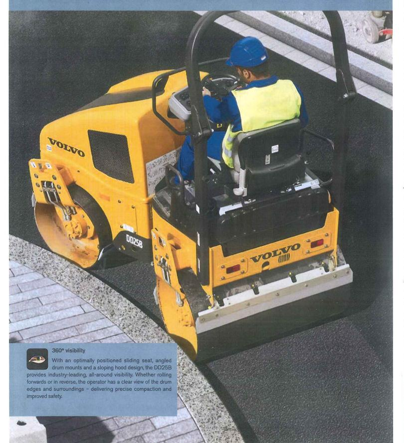
Introducing the DD25B, a highly efficient double drum compactor designed to increase performance and reduce fuel consumption on small scale compaction projects. Featuring the new Volvo D1.7A engine, this machine meets the strict Stage IV/ Tier 4 Final emissions regulations without adding an exhaust after-treatment system. Experience increased machine performance and enhanced productivity with Volvo.
