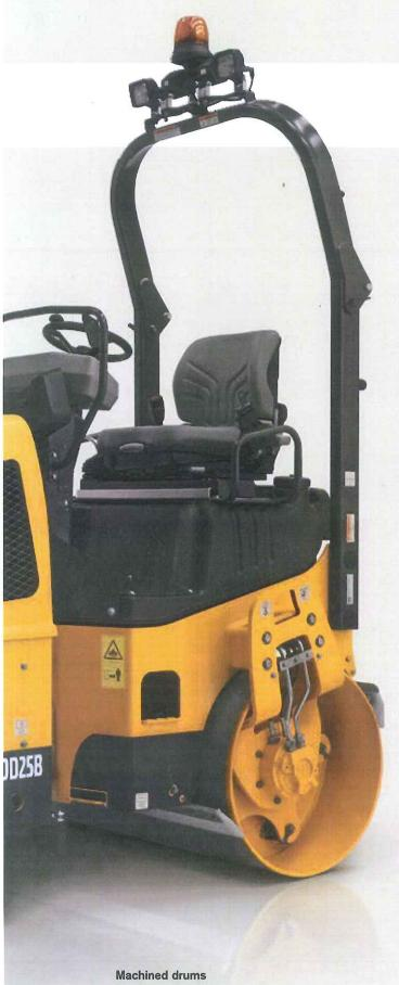
Machined drums with chamfered edges are perfectly round in order to produce a smooth, mark-free mat.
