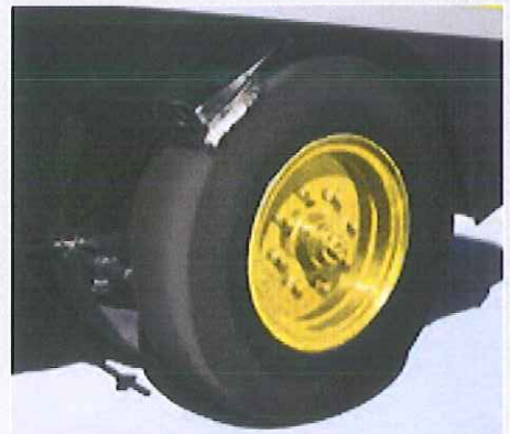
Cocoa mats on each tire help eliminate material pick-up
