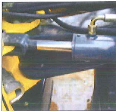
Bolt-in heavy duty oscillating / articulating centerjoint with 6.7 inches offset provision.
