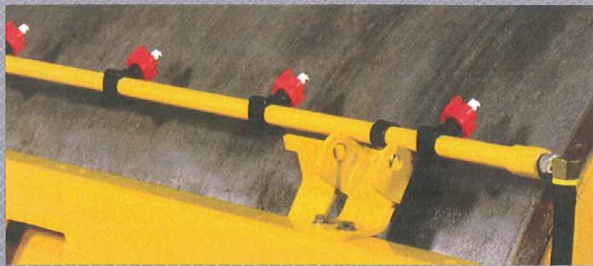
Front and rear nozzles optimize drum coverage
