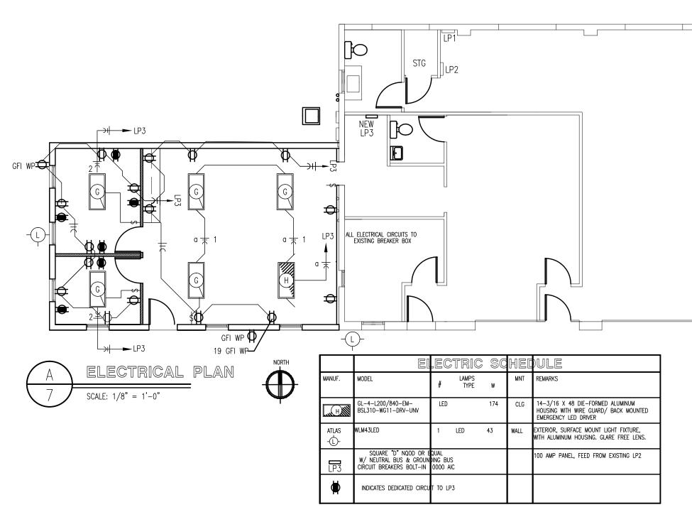
ELECTRICAL FIXTURES AND EQUIPMENT ARE SCHEDULED BY MANUFACTURER AND MODEL NUMBER FOR DESIGNINTENT ONLY. APPROVED EQUALS MAY BE SUBSTITUTED
