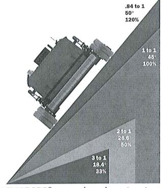
A **SLOPE-PRO**® can work on slopes too steep for a person or a ride-on mowers and without requiring track spikes or winch lines.
