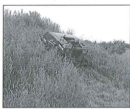
The **Slope-Pro**® is an industrial mower that is ideal for maintaining steep slopes or other hazardous locations, preventing the re-growth of
