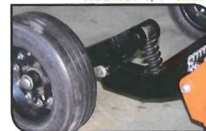
5615 Axles (spring axle) independent suspension
