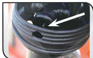
End cap grease zerk on PTO shaft
