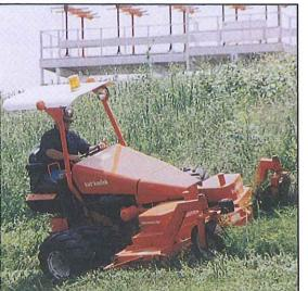
Tilting Suspension Seat with Restraining Arms — Tilting as much as 30 degrees as necessary for the operator to maintain his seating when traversing and turning on grades up to 40 degrees. Adjustable for operator weight, from 100-264 lbs.
