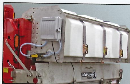
LS4T (tailgate mount 105 gal. poly reservoir)
