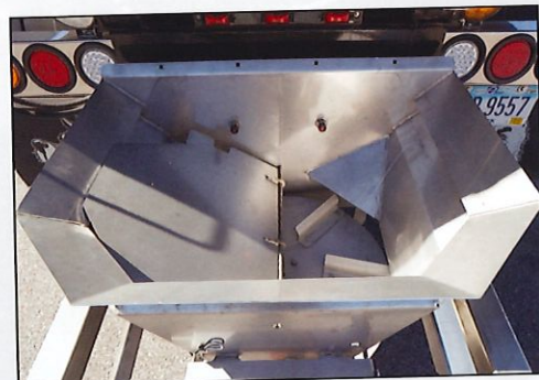
"hex flow" spinner assembly for optimal spread pattern
