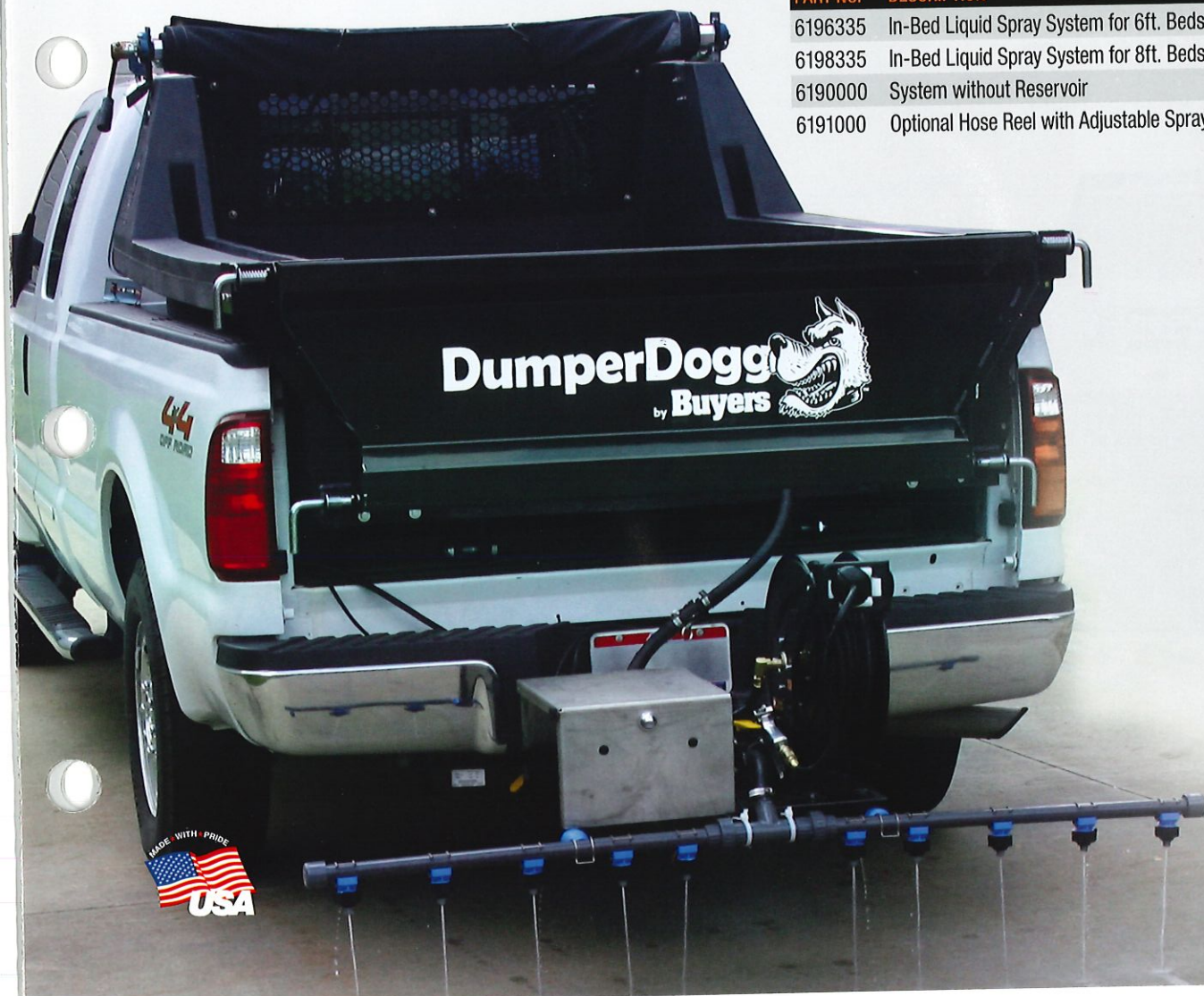
adjustable spray nozzle - pressure switch activates pump on demand
