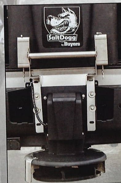
High flow chute with 14" spinner, open trough, and shield
