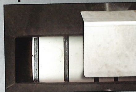
12" wide all steel pintle chain conveyor with stainless steel trough
