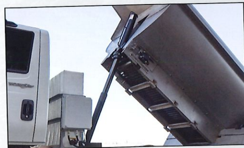
designed with a 3-stage, double-acting, front trunnion-mounted hoist
