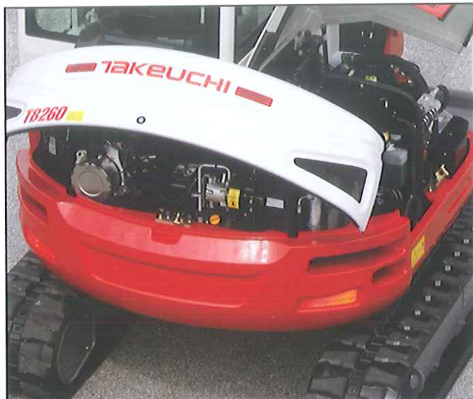
Large doors provide easy access to all major engine and hydraulic components.
