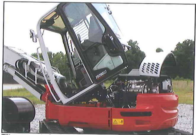
Tilt-up operator's platform provides improved access to all major hydraulic components.
