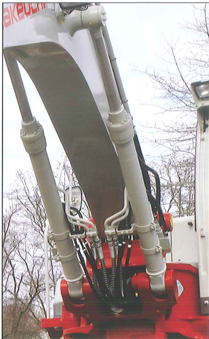
Two boom cylinders provide the strength needed for lifting, while the independent boom swing allows both excavators to dig offset over the left or right track.
