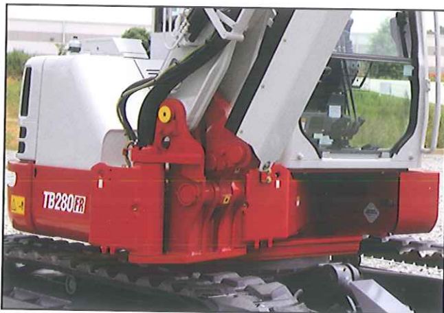
Unique Side-to-Side (STS) boom design enables this machine to work in confined work spaces.
