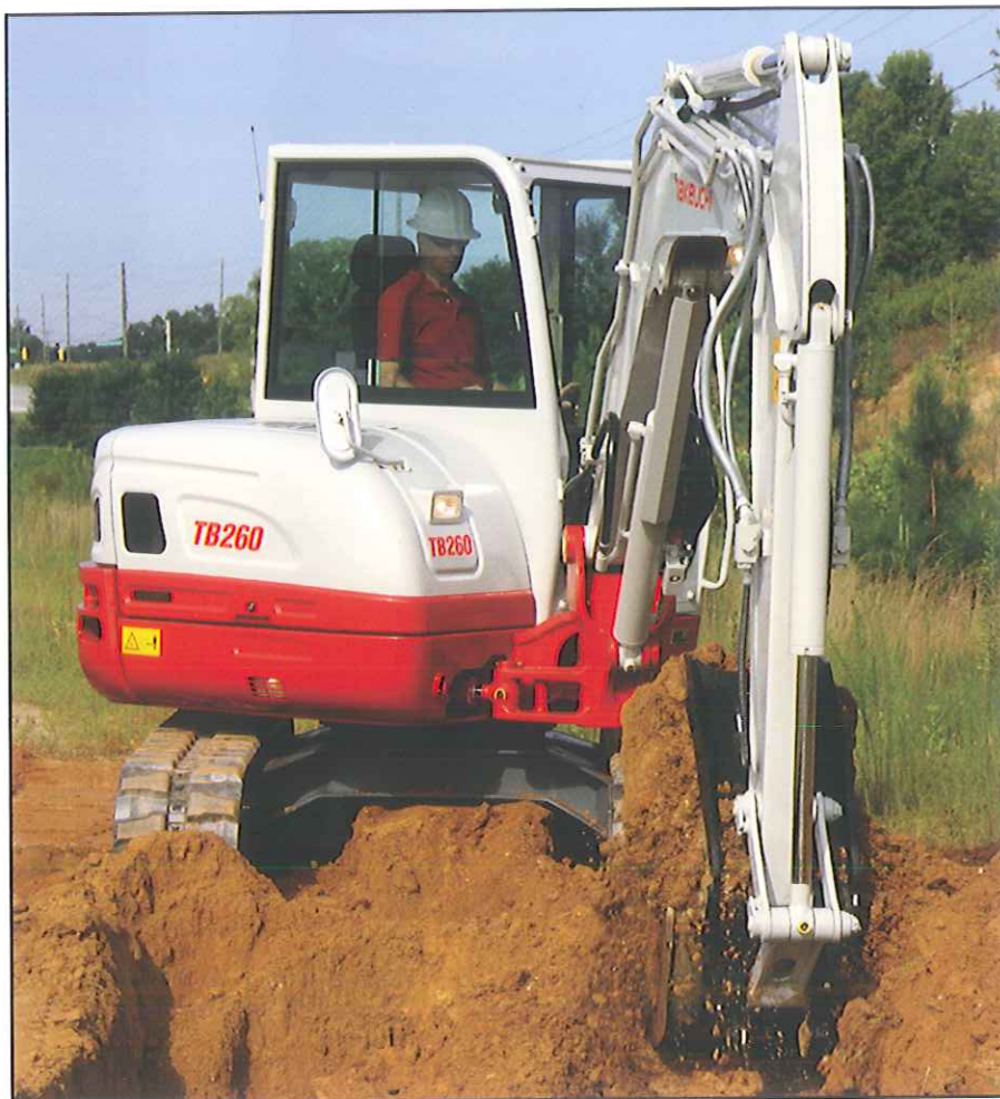
Low effort pilot controls and simple switches are easy to use.
