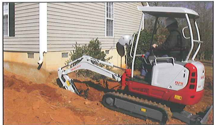
Standard long arm allows for greater reach and less time repositioning.
