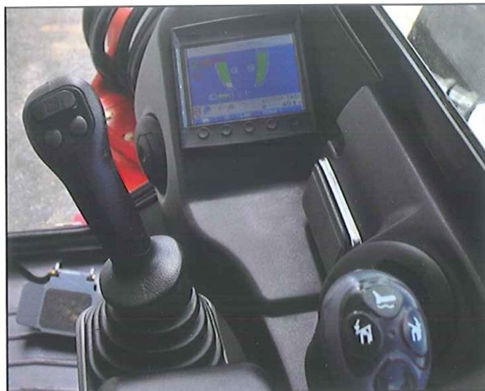
Low effort pilot controls and simple switches are easy to use.
