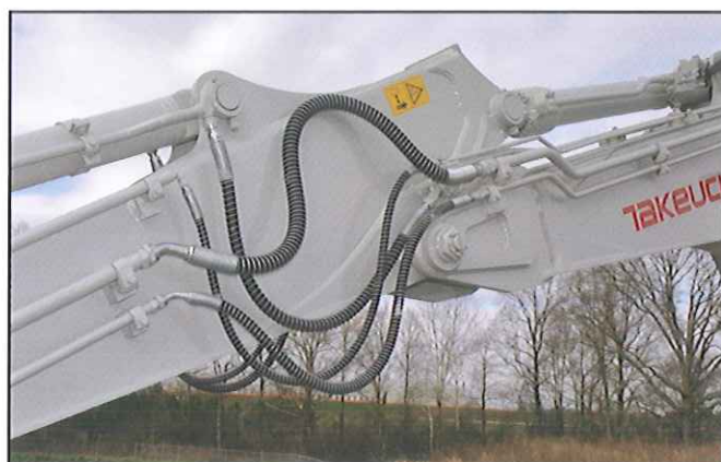
Both the TB290 and TB1140 have primary and secondary circuits with independent proportional control.
