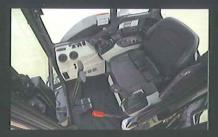
Proportional auxiliary hydraulics joystick with thumb toggle puts precision at your fingertips.
