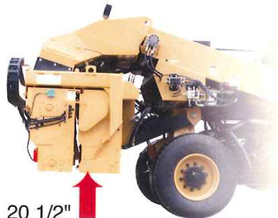
Variable height front hopper. Raise and lower hopper to clear obstacles. Easier loading.
