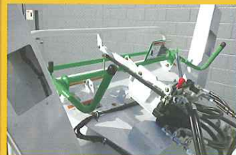
Panic bar and combination panic bar/feed control valve
