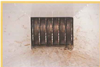
6" x 10" chipper opening to accept forked branches
