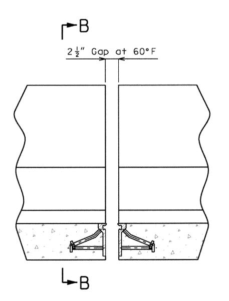
PART ELEVATION OF BARRIER CURB Note: Strip seal gland not shown for clarity.
