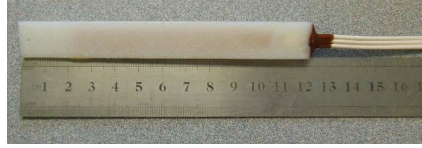
Figure 1 - Embedded strain gauge for monitoring shrinkage deformation
