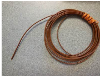
Figure 2 - Thermocouple used for concrete temperature measurement
