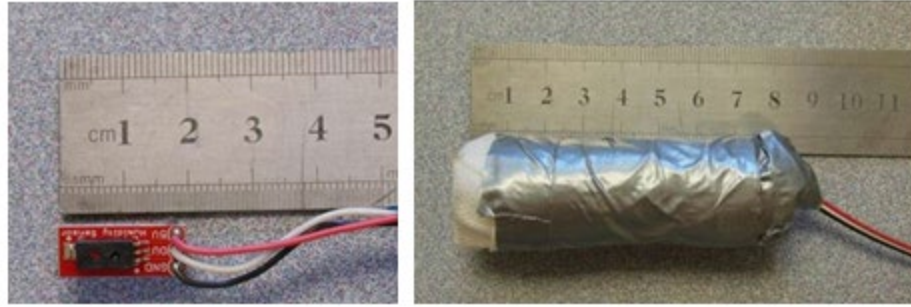
Figure 3 - Encapsulated relative humidity sensor before embedment in concrete
