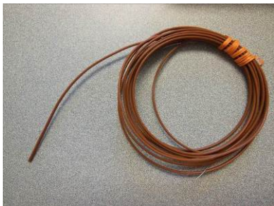
Thermocouple used for concrete temperature measurement
