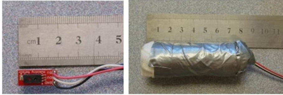
Figure 3.3. Encapsulated relative humidity sensor before embedment in concrete
