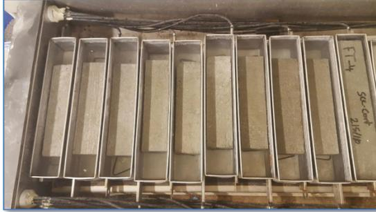
RCC Specimens Prior to Freeze-Thaw Testing
