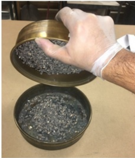
Figure C-14: Pennsylvania aggregate retention test: (a) the pan containing emulsion and aggregate was cured at ambient temperature for 24 hours, and (b) the pan containing the seal coat was inverted to allow the loose aggregate particles to fall. These aggregate particles were weighed to determine the initial loss in grams.
