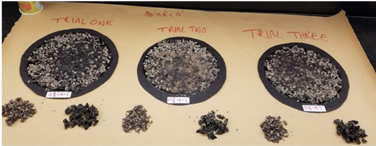
Figure C-4: Sweep test of specimens with 50% rubber: (a) 0.25" < R < 0.375" , and (b) 0.375" < R < 0.50"
