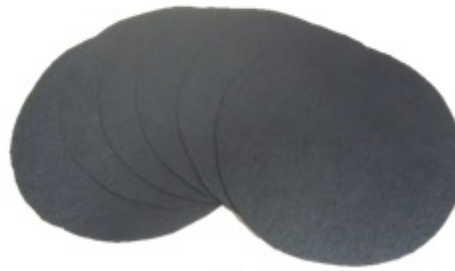
Figure C-2: Sweep test equipment (a) holding pan and brush holder, (b) specimen compactor (c) testing apparatus set-up, and (d) standard asphalt felt disks
