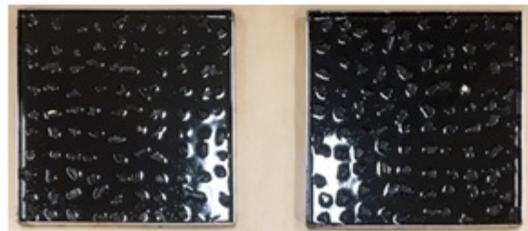
Figure C-8: Preparation of Vialit test specimens (a) prepare a clean and dry testing plate, (b) apply 79g asphalt cement emulsion, (c) emulsion after being tilted back and forth, (d) Placing aggregates uniformly using a 10x10 matrix, and (e) specimens with trap rock or crumb rubber
