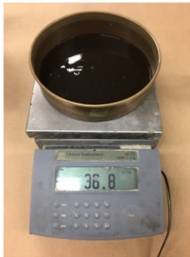
Figure C-11: Pennsylvania aggregate retention test: (a) preparing 300g of aggregate to obtain a single particle layer in 8" diameter pan and equivalent volume was used for the rubber that was 100 grams, and (b) 36.8 g of emulsified asphalt at 60 °C was applied inside an 8" diameter pan.
