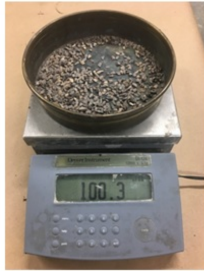
Figure C-14: Pennsylvania aggregate retention test: (a) the pan containing emulsion and aggregate was cured at ambient temperature for 24 hours, and (b) the pan containing the seal coat was inverted to allow the loose aggregate particles to fall. These aggregate particles were weighed to determine the initial loss in grams.
