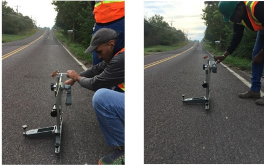
Figure 41: Field skid resistance test for a segment
