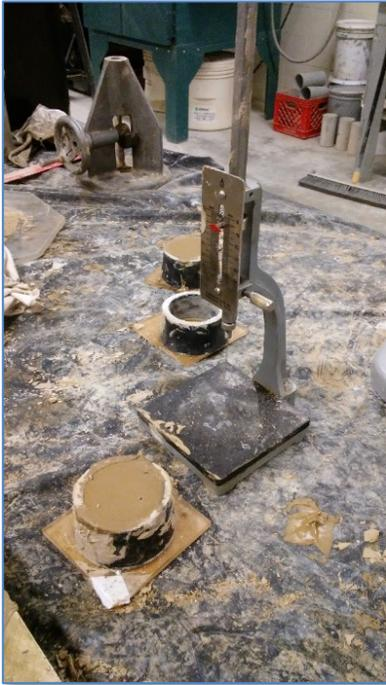
Setting time testing of zero-cement mortar
