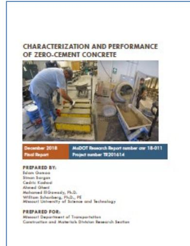
This study revealed that ZCC can be used as a replacement for CC. ZCC showed good workability and adequate compressive strength for structural applications ranging from 3,660 psi to 7,465 psi based on the curing regime and source of FA. Some ZCC mixtures successfully passed 300 cycles of freeze and thaw per ASTM C666-15 procedures A and B.
