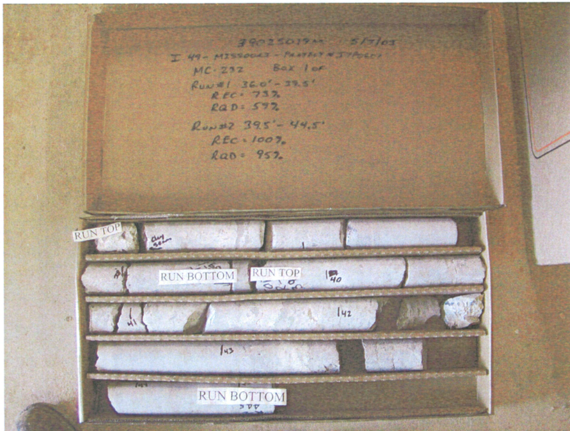
I 49 Missouri Missouri J7P0601 Boring MC-229 Run No. 1 36.0 Feet to 39.5 Feet Run No. 2 39.5 Feet to 44.5 Feet
