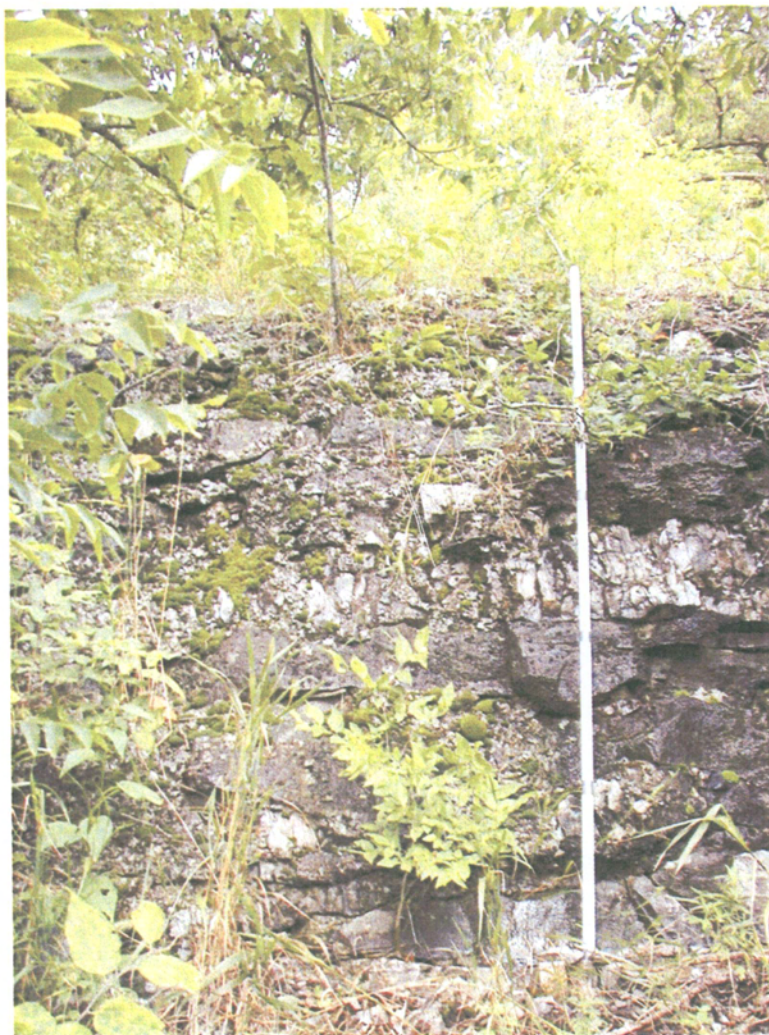
Photo 10: Rock outcrop near middle of exposure, below MC-18. Shown are interbedded chert and limestone beds. This exposure is located approximately 30 feet south of the basal outcrop shown in Photos 1 through 3. The top of this outcrop is at a similar elevation as the top of the basal outcrop. Jacob staff is 5 feet long with 1-foot divisions (gray) for scale.
