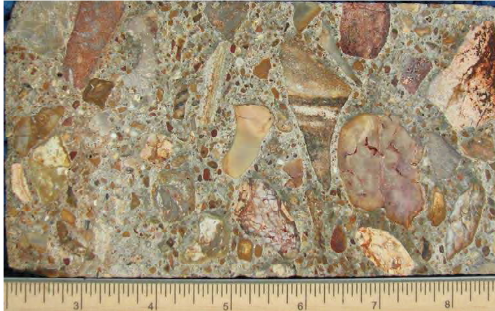
Figure 7: Photograph showing the good condition of Core SV-3. The outer surface is to the left. Scale in inches.
