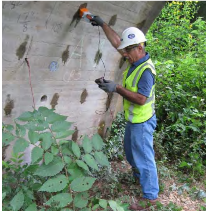
Photo 7: Half Cell Potential Testing
