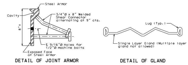
**Table of Allowed Transverse Strip Seal Expansion Joint System**
