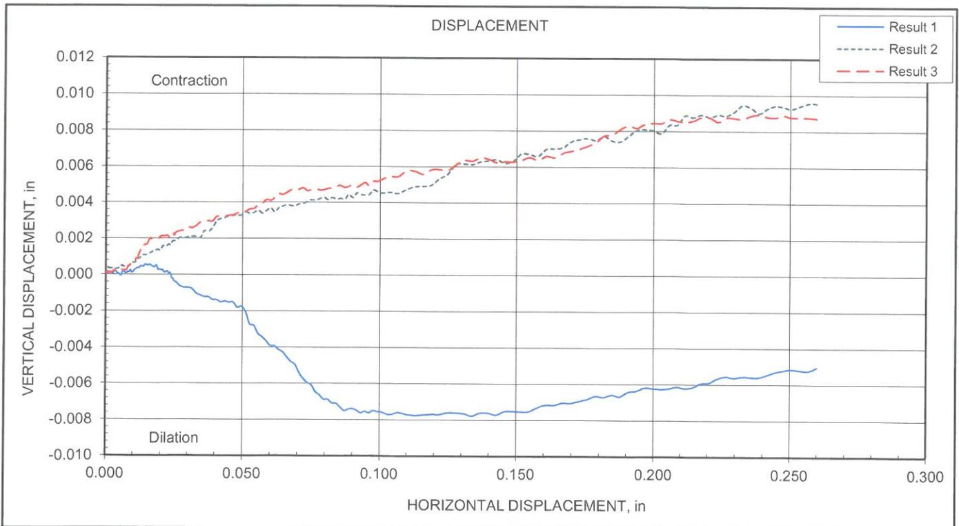
**DIRECT SHEAR TEST OF SOILS UNDER CONSOLIDATED DRAINED CONDITIONS
