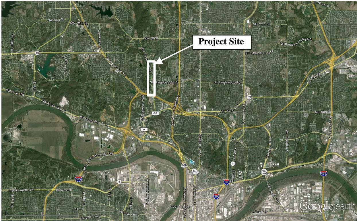
The project will consist of widening Waukomis Drive from the exit ramp of northbound I-29 to approximately 1400 feet north of NW 62<sup>nd</sup> Street. This project includes widening the existing two-lane roadway, extending the box culverts at two creek crossings, and stabilizing the stream banks of the two creeks.
