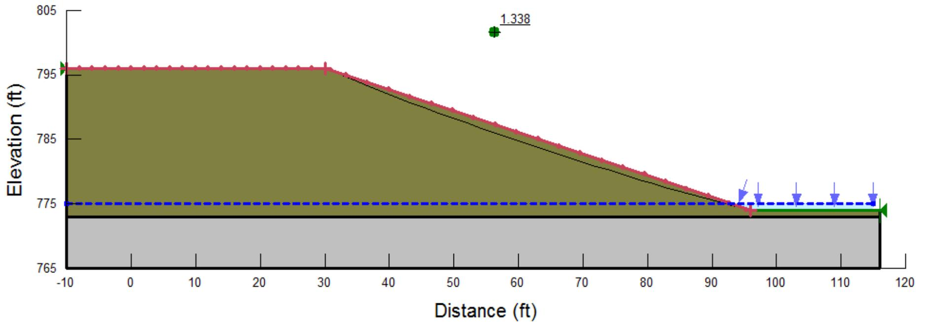
Figure 2: Waukomis 3.0H:1.0V Slope Drained
