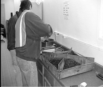
Splitting the loose mix sample taken from the road - four samples
