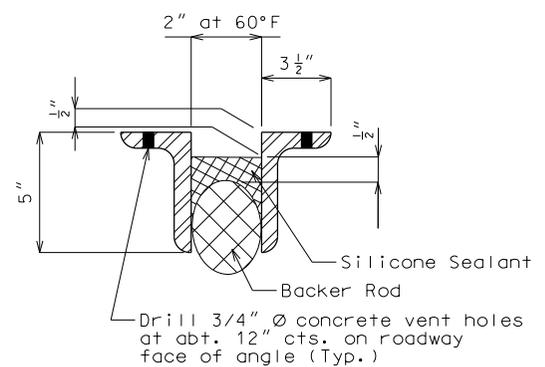
Minimum thickness of angle shall be 1/2".
