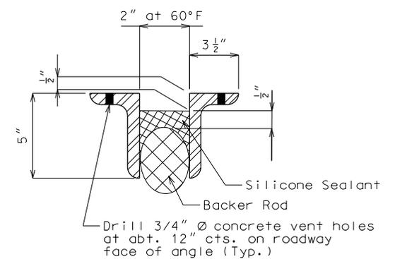
Minimum thickness of angle shall be 1/2".
