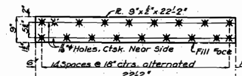
CAP PLATE AT END BENT
