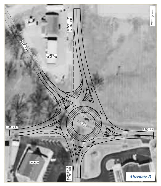
*Alternate B Details* With this alternate, County Road 448 or Miller Road will remain part of the intersection.
