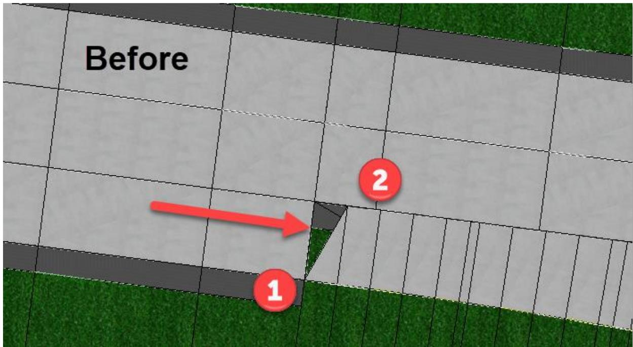
The first two Template Drops for Ramp 2 are both solving for the Route 50 EOP. The first Template Drop is solving for the widened Axillary Lane EOP, and the Second Template Drop is solving for the normal Route 50 EOP.
