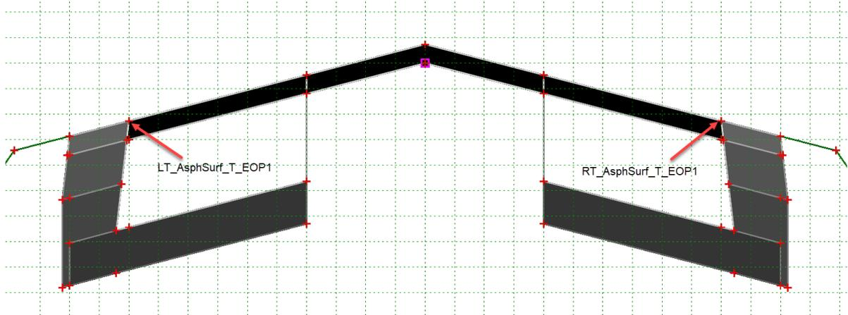
To get the Widening to stop at an offset of 12' from the baseline we will need to modify the **Big Horn - Match Existing Slope Surface Course** Template. To do this select the **RT\_AsphSurf\_T\_EOP1** and the **LT\_AsphSurf\_T\_EOP1** points and modify the **Horizontal Constraint** to have a parent point **AsphSurf\_B\_CL** with an **Offset = 12 ft**
