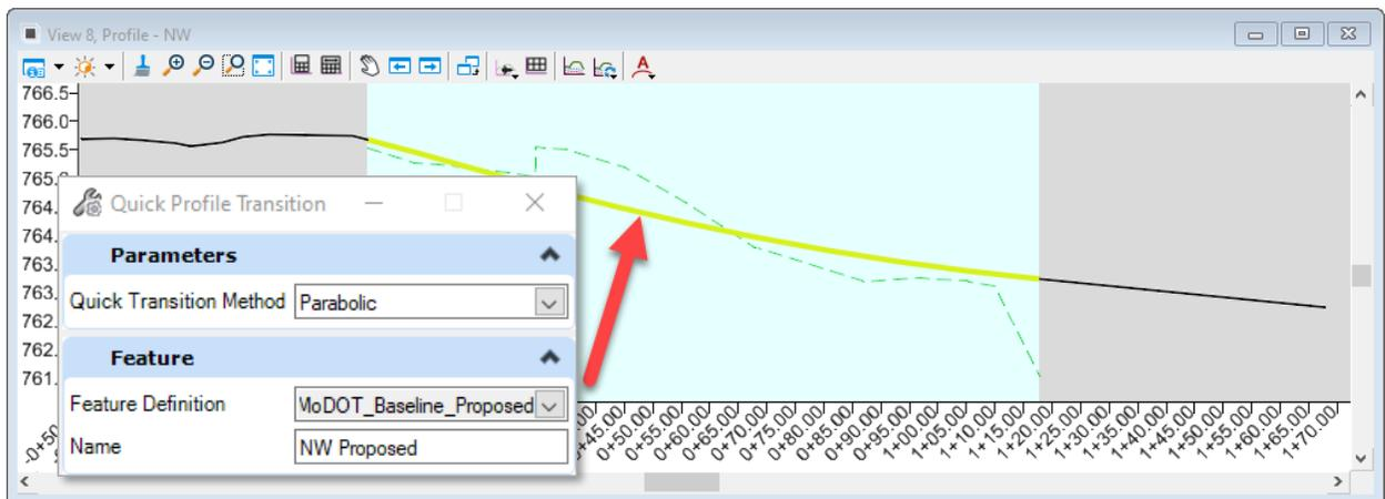
**Note:** The **Quick Profile Transition** tool will automatically make the newly created profile Active.
