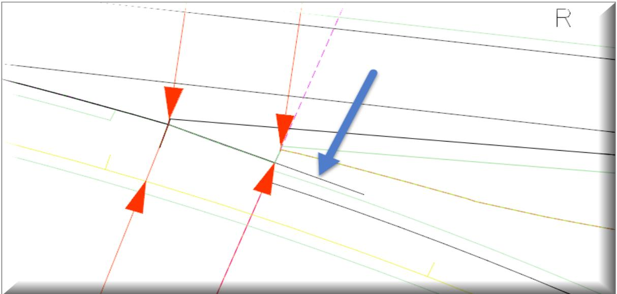
68) Edit the J5P0555\Ramp2\Ramp2 template and modify the **Horizontal Constraint** for the **LT\_Conc\_T\_EOP** point to a width of **18'**.
