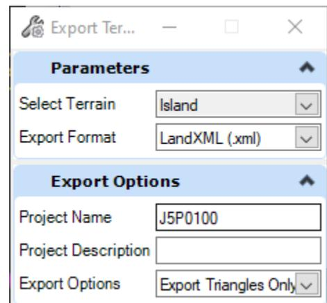
70. Once exported, delete the **Island Terrain** in the **Corridors\_J5P0100.dgn** file. Also switch the **Linear Template Feature** back to **1-Final x 1**.
