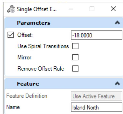
80. Repeat the **Single Offset Entire Element** tool for the **SW Radius Return**. Offset the line toward the intersection.
