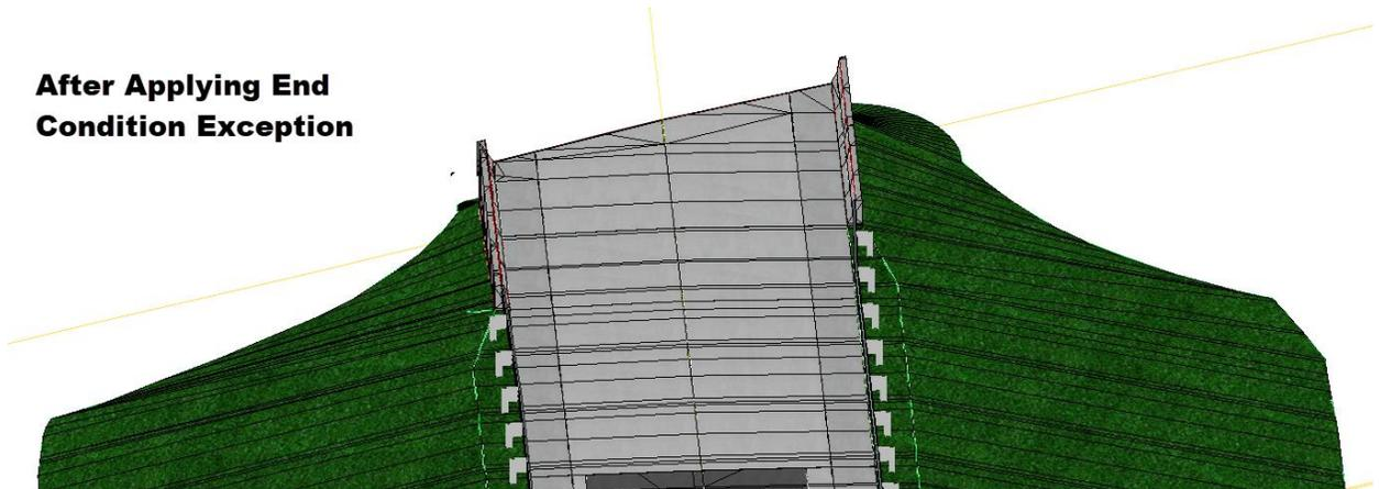
50) To help close the gap near the start of the Barrier on the left side of the roadway, add a **Key Station** at **71+97.88**
