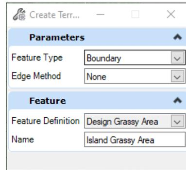
For *Locate Element to Add*, **Left-Click** the 3D line along the top inside edge of the curb (**Curb\_Surf\_Back**).
