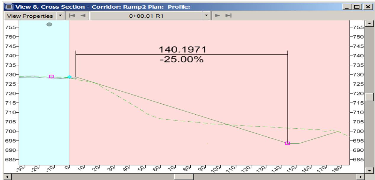
**Note:** There is one section off the **Route 50 Corridor** that does not solve for a Ditch after applying the adjusted Point Controls. To make that section solve as a ditch, the User could move the **Special Ditch Profile** down one foot at the start the profile.
