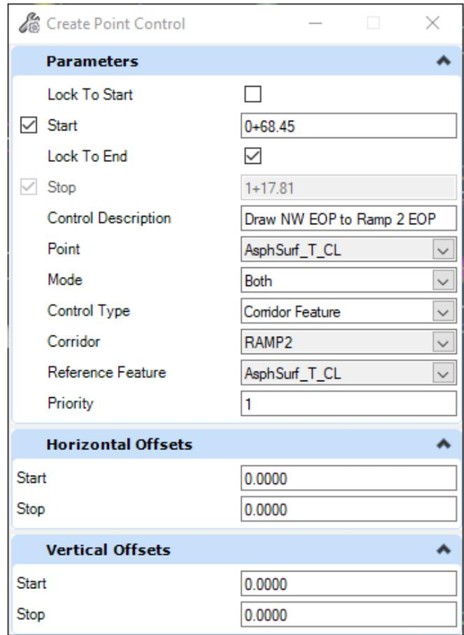
57. **(Individual Step)** Using the same steps in storing the **NW Linear Template**, that drew the **NW EOP** up to the **Ramp 2 EOP**. Create a **Point Control** for the **SW Radius Return** that does the same thing.
