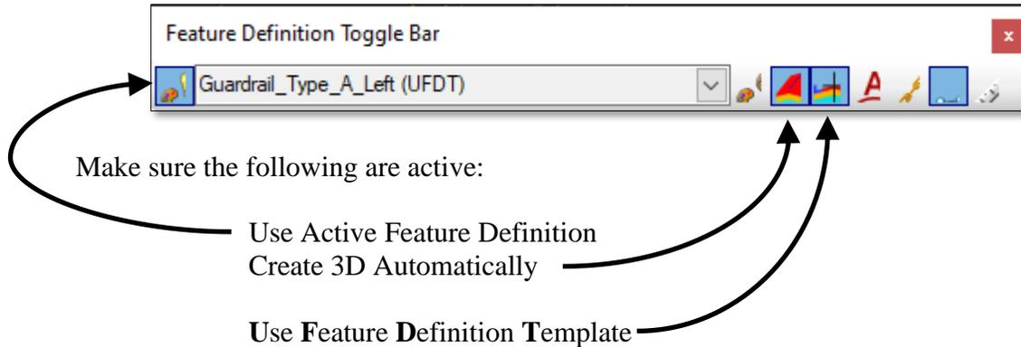
43) Using the **Horizontal Geometry - Variable Offset Taper** along with **Civil AccuDraw** tool, place on **BOTH** Left and Right sides of the roadway the 1ft offset taper section of the guardrail.
