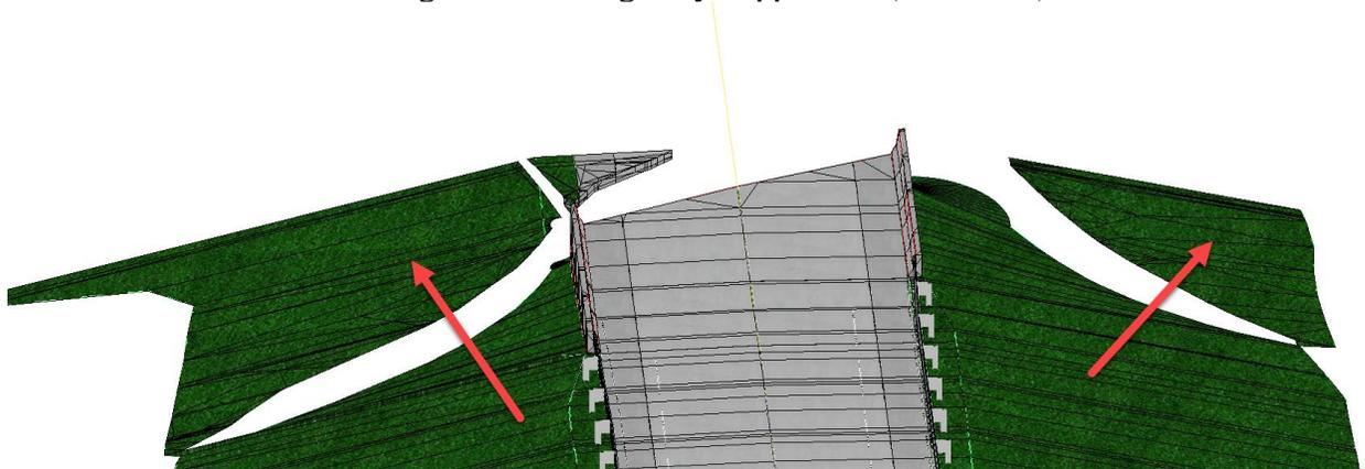
To remove the two slopes we are going to apply a **End Condition Exception** to the Mainline Corridor for each side of the roadway.
