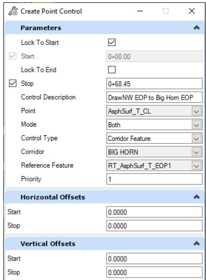
55. **(Individual Step)** Using the same steps in storing the **NW Linear Template**, that drew the **NW EOP** up to the **Big Horn EOP**. Create a **Linear Template** and then a **Point Control** for the **SW Radius Return** that does the same thing. (These steps started back on step 51).
