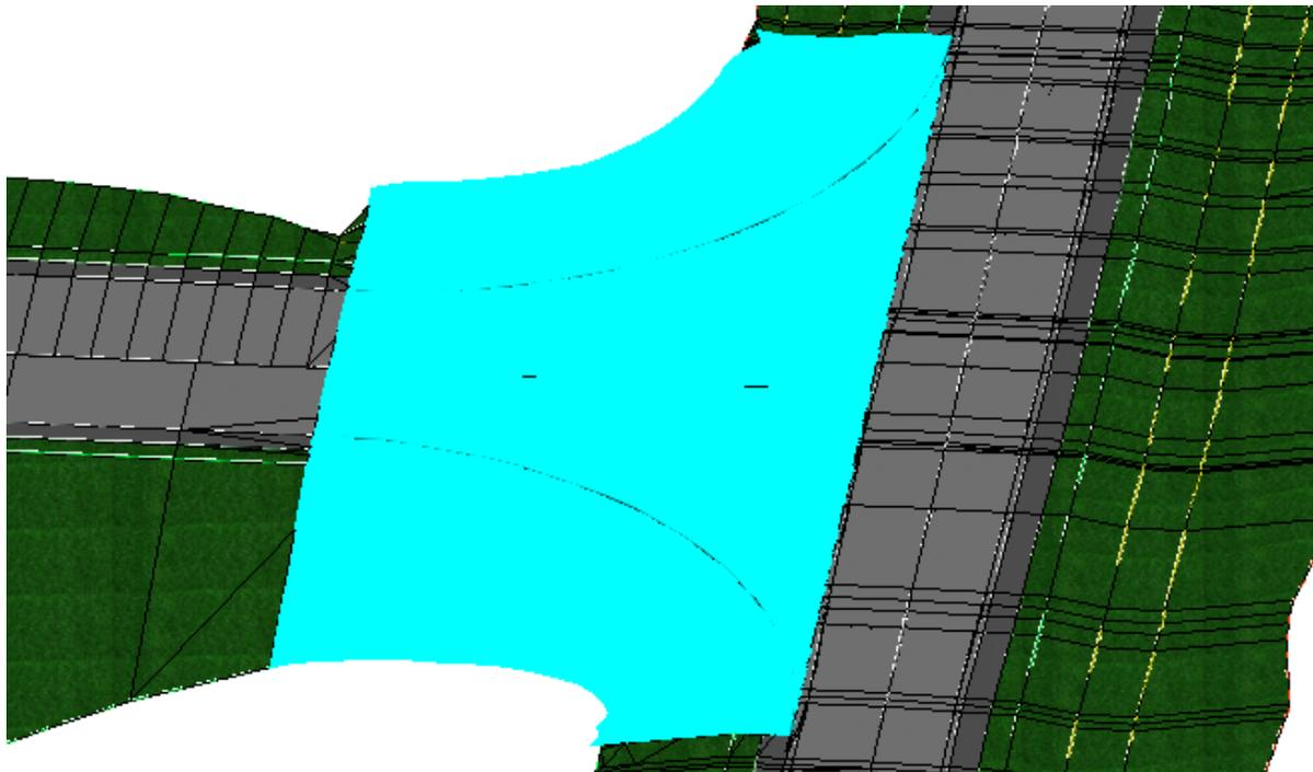
64. To create the Terrain, select the **From Elements** tool by selecting the **OpenRoads Modeling Workflow** → **Terrain Tab** → **Create Section**.
