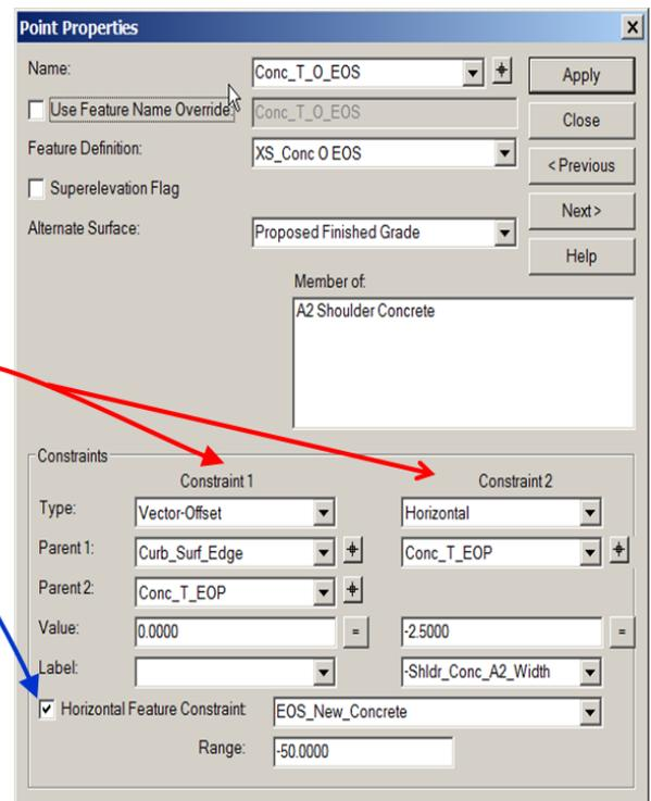
67) Add the **EOP\_New** line that transitions from an **18'** offset to a **20'** offset as corridor references in the **Ramp2 Corridor**. The EOP line is near the grass gore point (see **Blue Arrow** below).
