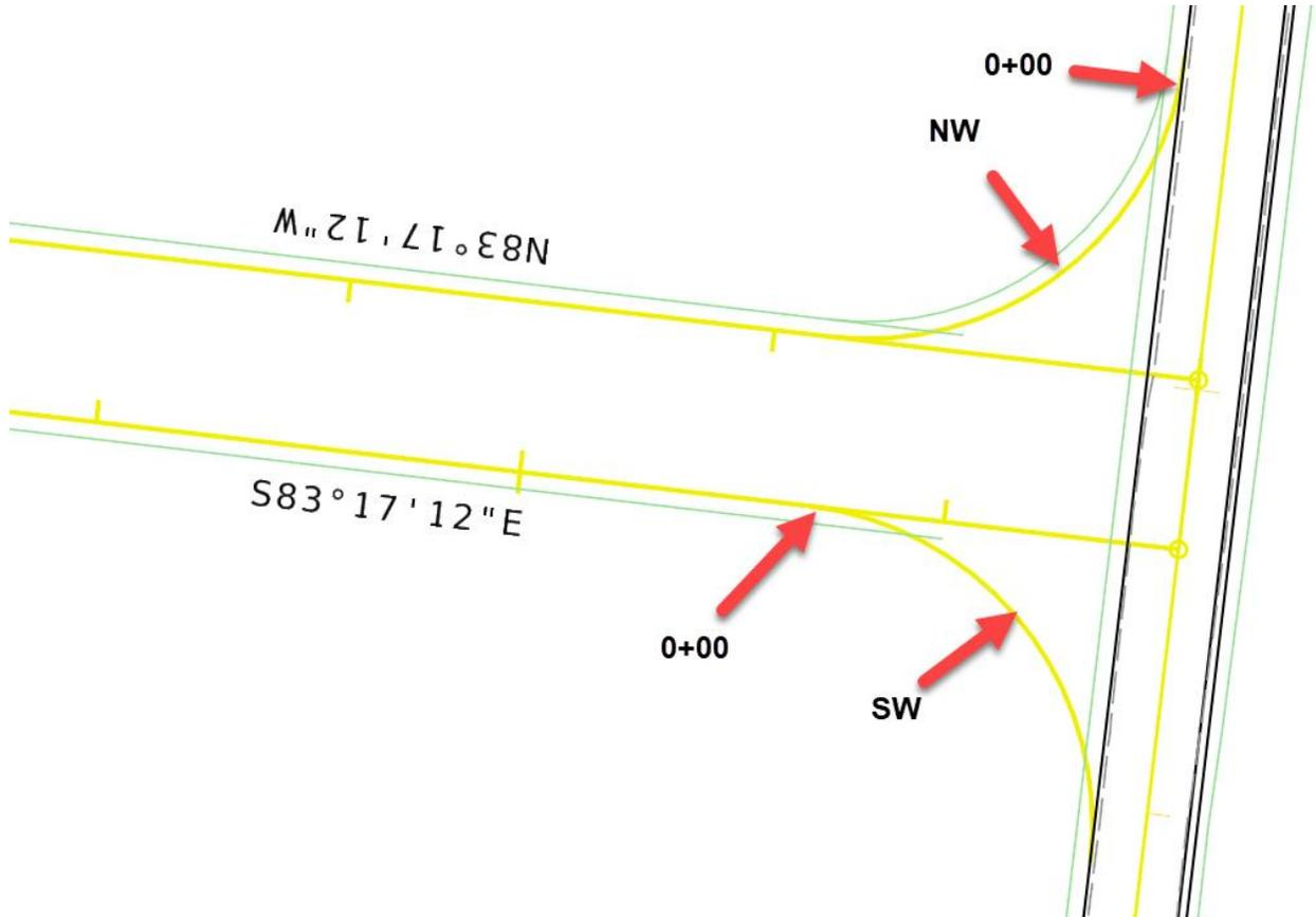
46. In the next few steps, we are going to define a profile for the Radius Returns based on the **longitudinal** slopes of the edge of pavements coming into each Radius Return.
