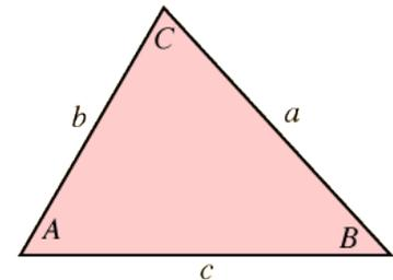
$$b = \left( \frac{\sin 75^\circ}{\sin 15^\circ} \right) (7ft) = 26.12ft, \text{ use } \mathbf{30ft} \text{ for Guardrail Widening Transition Distance.}$$
