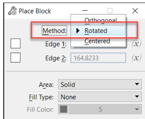
f. Create **two** blocks. One up-station and one down-station using the copied offset lines by using a keypoint snap to each end of the extended line. You will want them to overlap.
