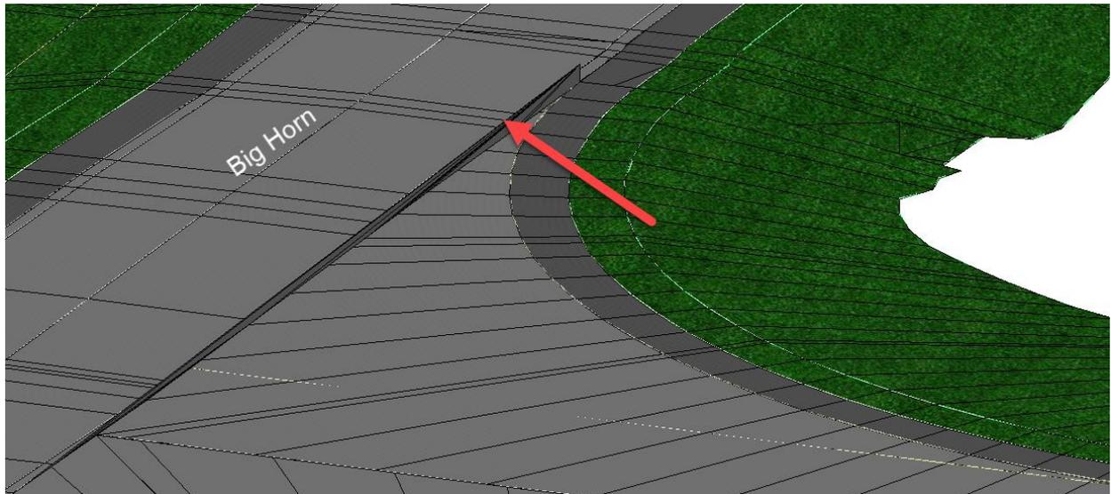
You may need to add a slight offset to the **SW Linear Template Point Control**. To do this select the **Corridor Objects** icon from the **SW Linear Template** heads-up tools.
