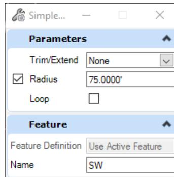
44. For the **NW Radius Return**, use the same **Simple Arc** tool with a radius of 75.
