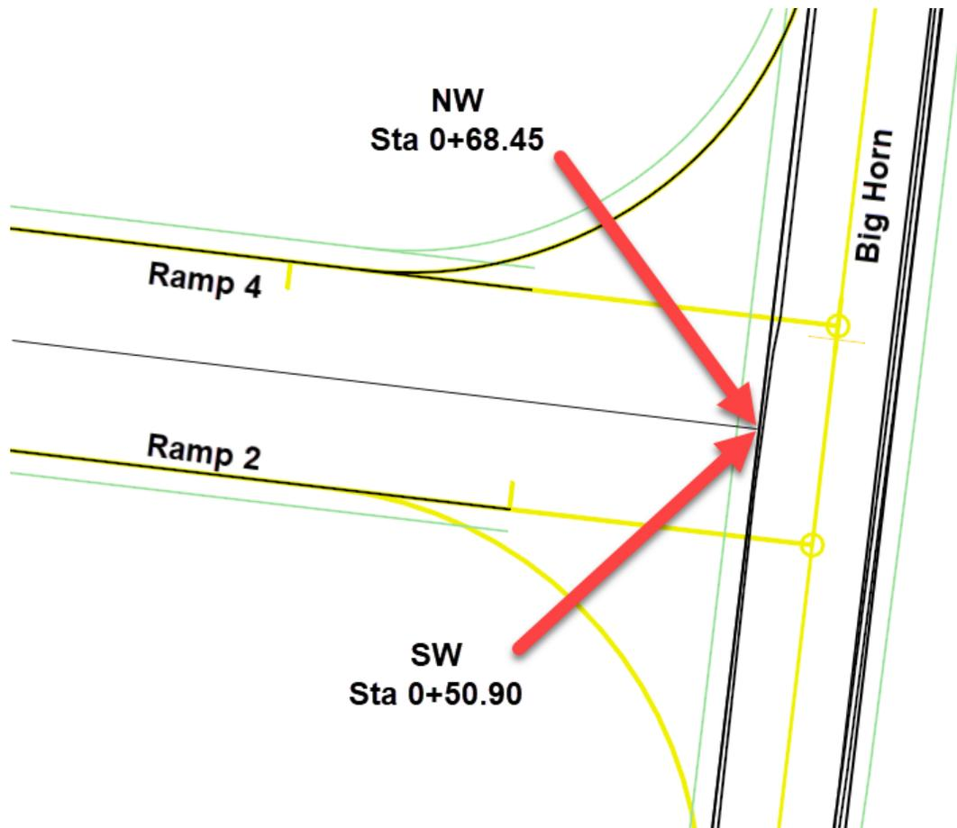
54. Using the heads-up prompts on the **NW Linear Template** grips, select the **Corridor Creation Tools** → **Point Controls**
