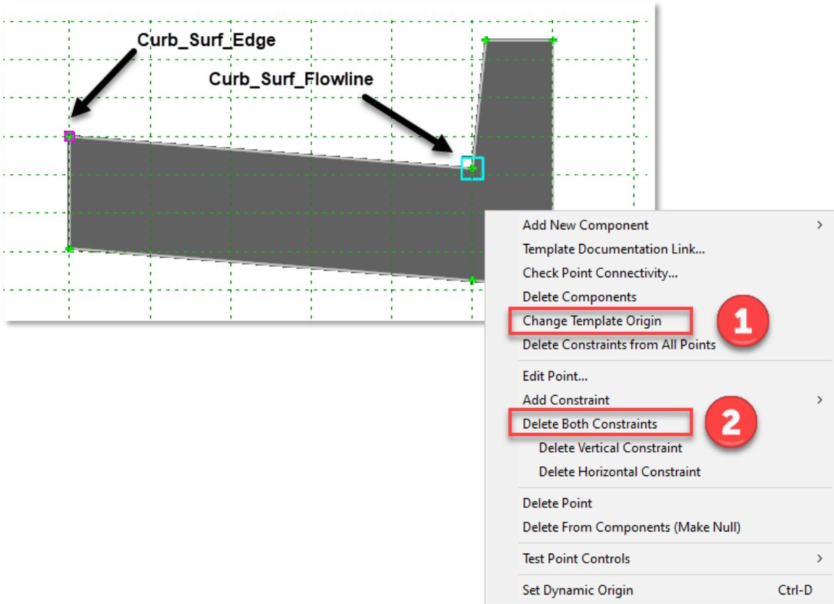
96. Zoom to the left of the template and locate the **Curb\_Surf\_Edge** point. **Double-click** on this point.
