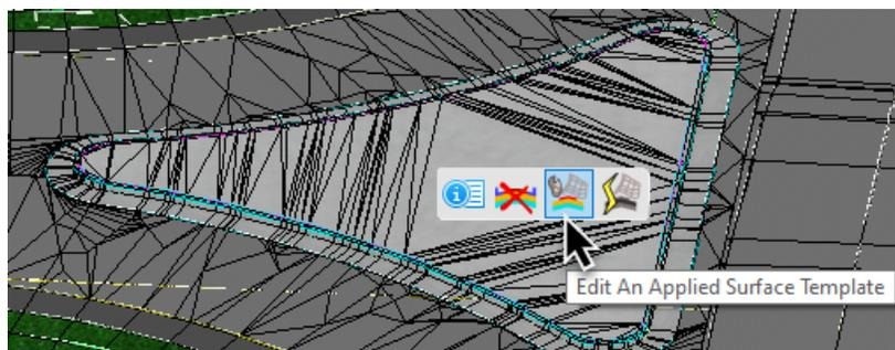
112. When the Template window opens select the **Active Template** Tab. Then open the **Parametric Constraints** folder and **right-click** on the **Pvmt\_Surf\_Conc\_Depth** and select **Edit**.
