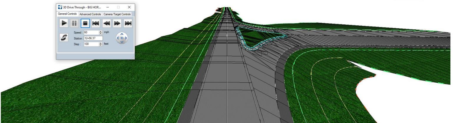
139. After using the 3D Drive Tool, you will notice a fish-eyed view within your 3D View, to turn that view effect off go into the **View Attributes** and deselect the “**Camera**” setting:
