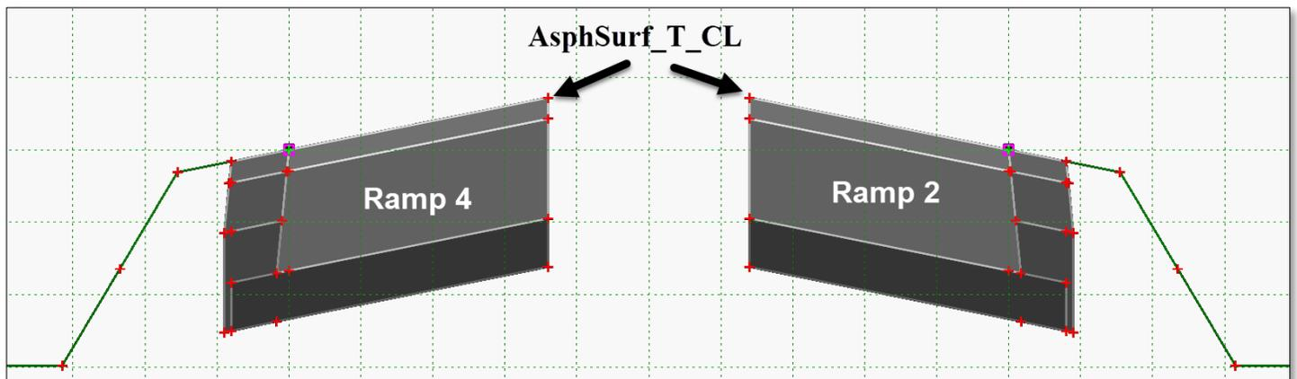
**NOTE:** There appears to be a problem with the **Ramp 2 Profile**. The **Ramp 2 Profile** is supposed to be designed so that the **Crown Point** in-between the **Ramp 2 and Ramp 4 Corridors** matches the elevation of the **Big Horn EOP/EOP** line. You can see in the 3D view that the **Ramp 2 Corridor** is diving too far below into the Big Horn Corridor.
