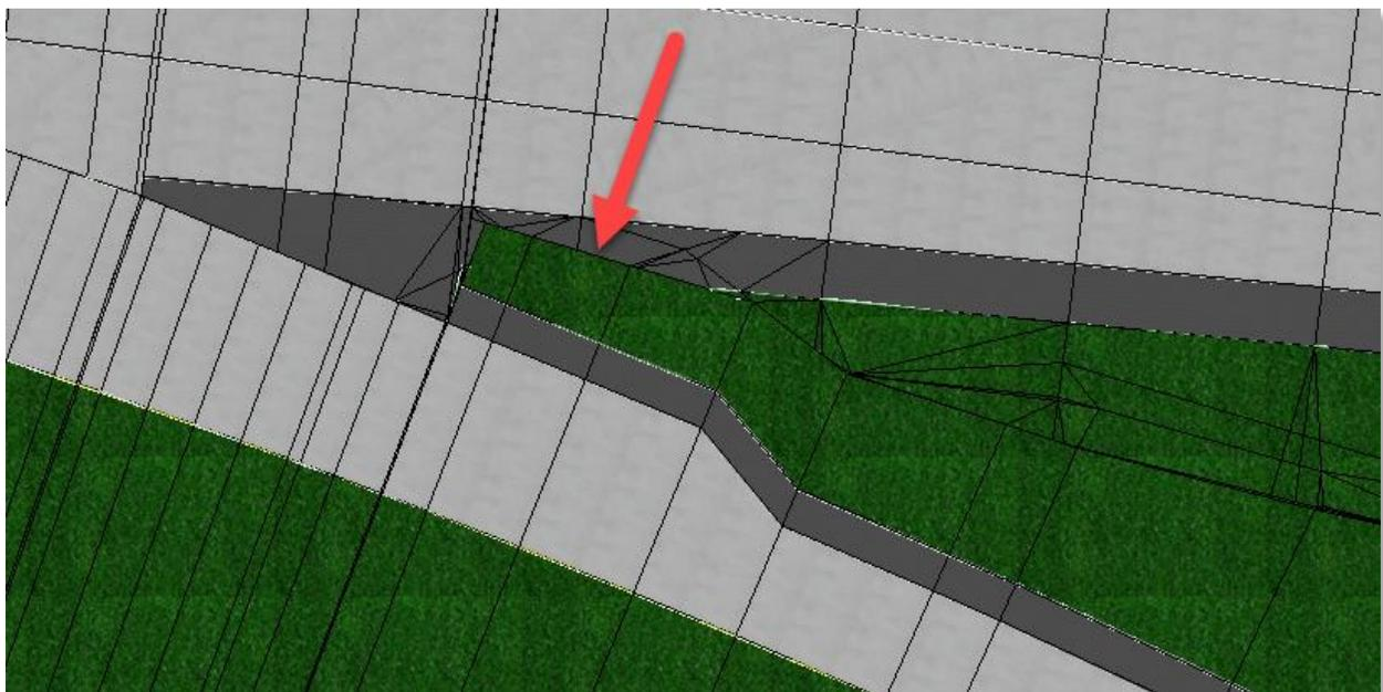
**Create Special Ditch - Drawing the Ditch Foreslope to a Alignment and Profile**
