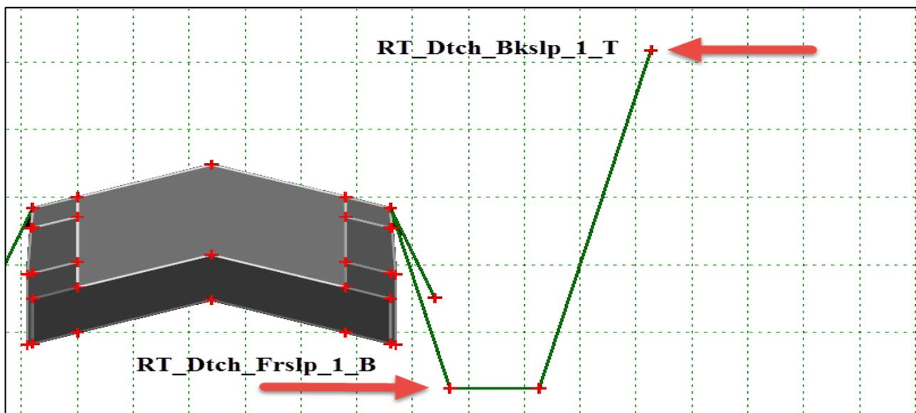
75) In the **Route 50** and **Ramp 2** Corridors, edit the Special Ditch Point Controls by changing the **Point Control Mode** from **Both** to **Vertical**.
