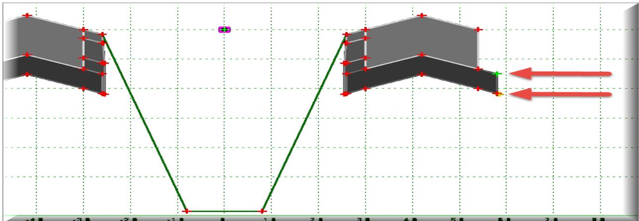
**Note:** The next few steps will add an **auxiliary lane** on the right side of the template. The auxiliary lane is being added to provide the User a way to transition over a distance the **Pavement Normal Slope** of (2%) to the slope at the beginning of **Ramp 2 (3.87%)**.
