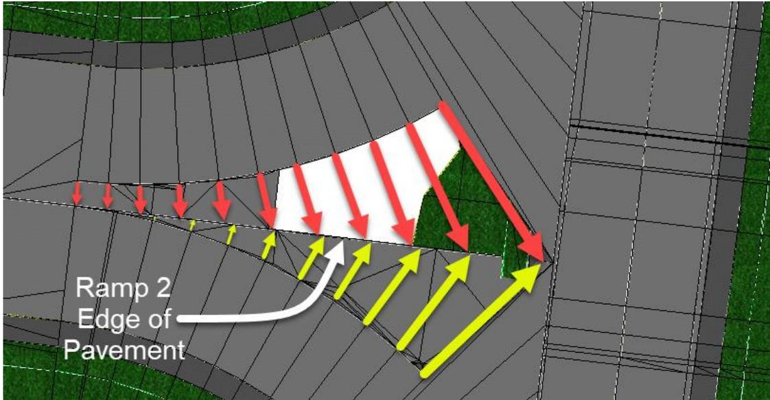
56. Using the heads-Up prompts on the **NW Linear Template** grips, select the **Corridor Creation** tools → **Point Controls**. Fill out dialog as indicated below:
