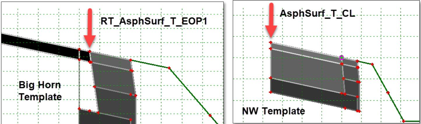
But first, another piece of information we will need for our Point Control is the **Start** and **Stop** Location for drawing to the **Big Horn Edge of Pavement**. With the NW Linear Template, we will start at **Sta. 0+00** and end at **Sta. 0+68.45**
