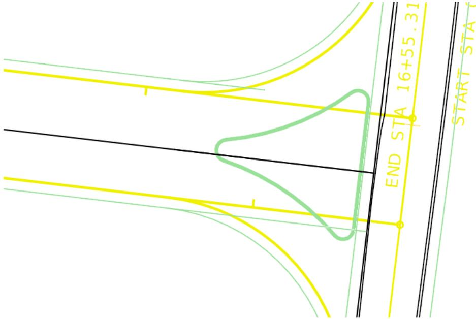
83. Next, we are going to **Create a Complex Element** around the island to make it one piece. To do this use the **Complex by Elements** tool located under the **OpenRoads Modeling Workflow** → **Geometry Tab** → **Horizontal Section** → **Complex Geometry** tools.
