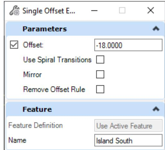
81. Repeat the **Single Offset Entire Element** tool, one more time, for the **Big Horn** baseline. Offset the line toward the **West** (away from the Big Horn centerline).
