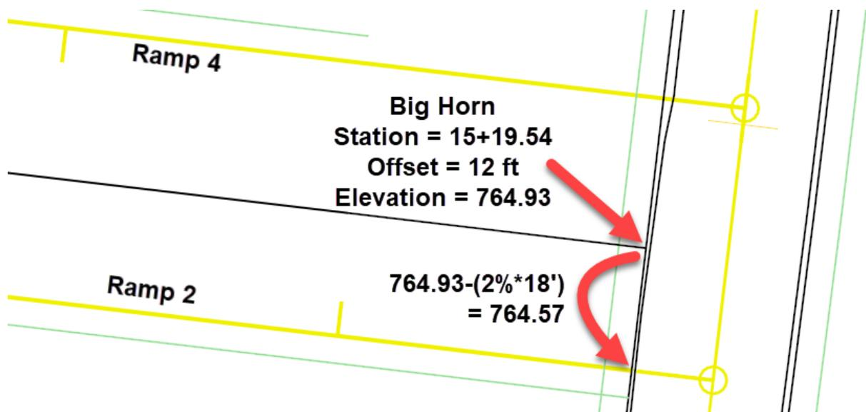
40. Open the **Corridors\_J5P0100.dgn** file to see the adjustments to the Ramp 2 Corridor modeling up to the **EOP/EOS** point of Big Horn.
