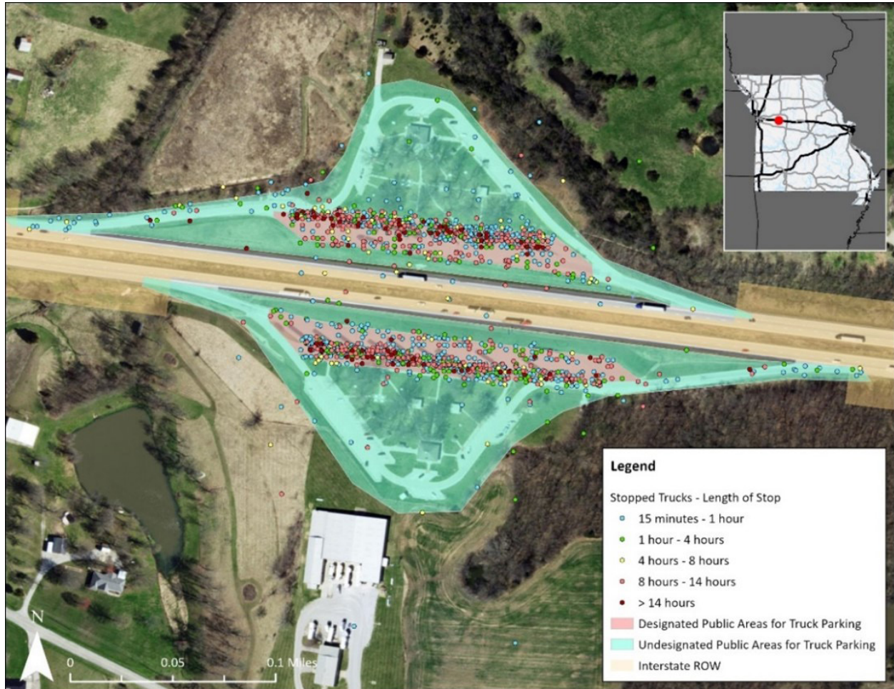
Figure 6 – Typical Public Truck Parking Facilities (Concordia Rest Areas) and Stops
