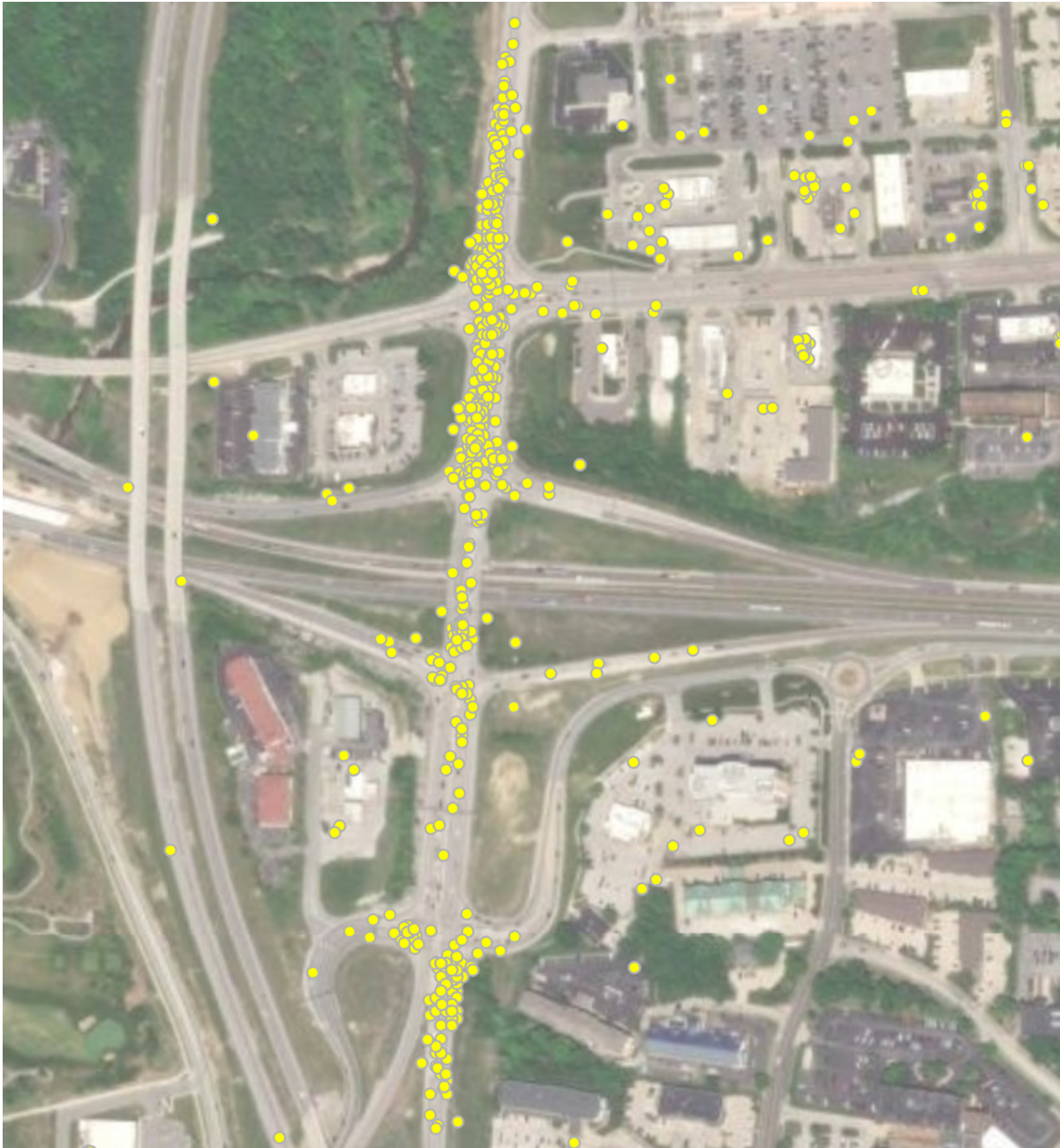
Figure 11 – Example Non-Facility Parking on Public Right-of-Way Without a Truck Parking Restriction
