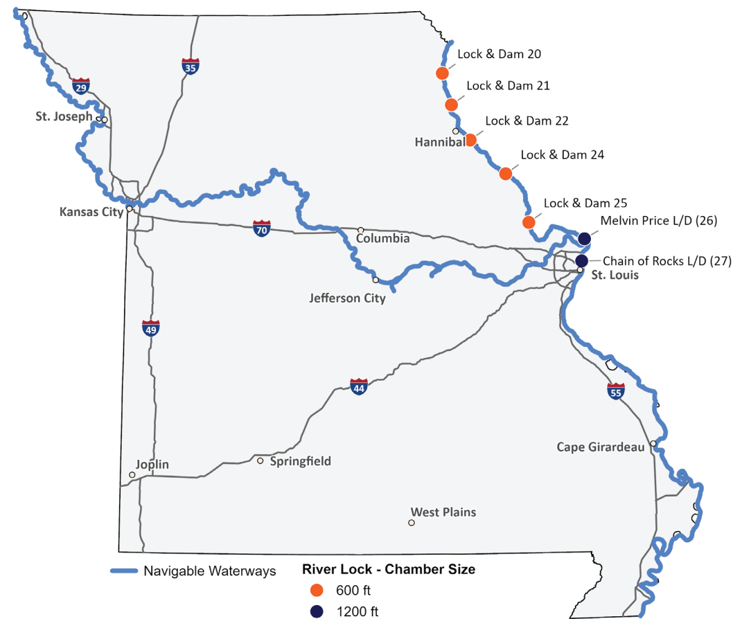
Figure 29 – Lock/Dam Locations and Lock Chamber Lengths
