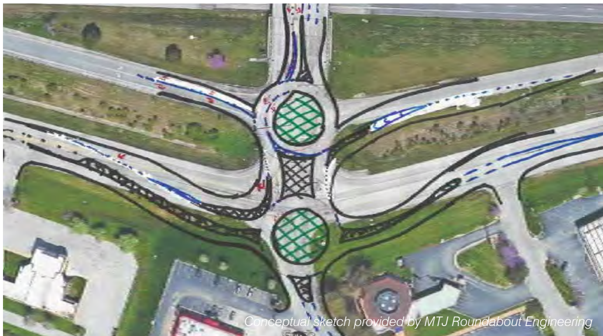
Exhibit 4-1 - Alternative 1 - Two Closely Spaced Roundabouts
